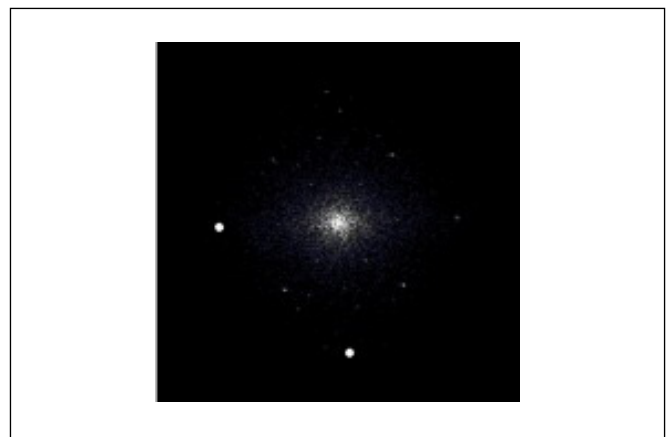
Figure 3. 2D-FFT spectrum of a paper sample image showing highlighted peaks used for CD shrinkage measurement. The peak close to horizontal axis was used for measuring the CD separation and the inclination of the MD yarns marks from machine direction. The peak close to the vertical axis was used to measure the deviation of wire CD yarns from cross-machine direction for compensation of possible misalignments of forming fabric during operation
