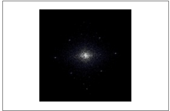
Figure 2. 2D-FFT spectrum in frequency domain obtained from the image of Figure 1 (zero-padded to 512 x 512 pixels before processing)
