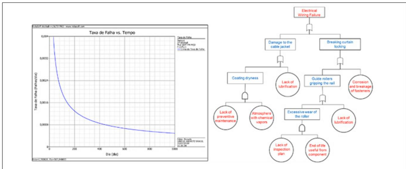
Figure 6. Swing conveyor's electrical wiring graph of Failure rate and Failure Tree Analyses
