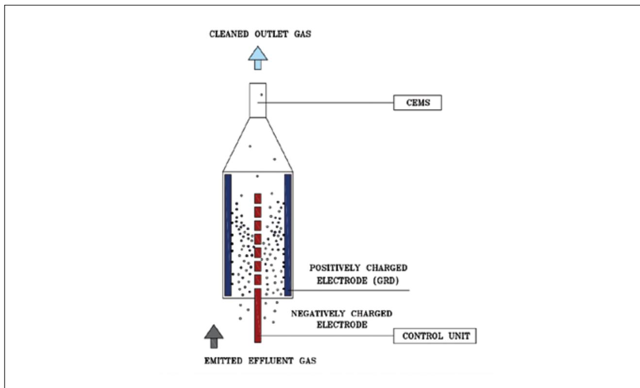
Figure 2. Representative flow pattern and electrode disposition
